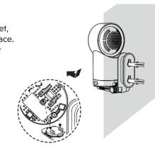
4. Place the baby unit on the wall mount bracket, and then slide it forward until it locks into place. Align the holes on the wall mount bracket with the screws on the wall, and slide the wall mount bracket down until it locks into place.
